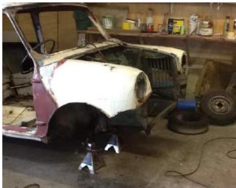
I have enclosed some before repair photo's and hope that members with rear sliding windows will notice what hidden damage can be found. The rust under the rear doors has been cut out and a special replacement section fabricated. Both A panels inside and out have been replaced, along with the lower front panel. In addition a lot of smaller areas have had to be repaired. I have replaced the front bearings, and bushes, and will strip the rear axles next.
